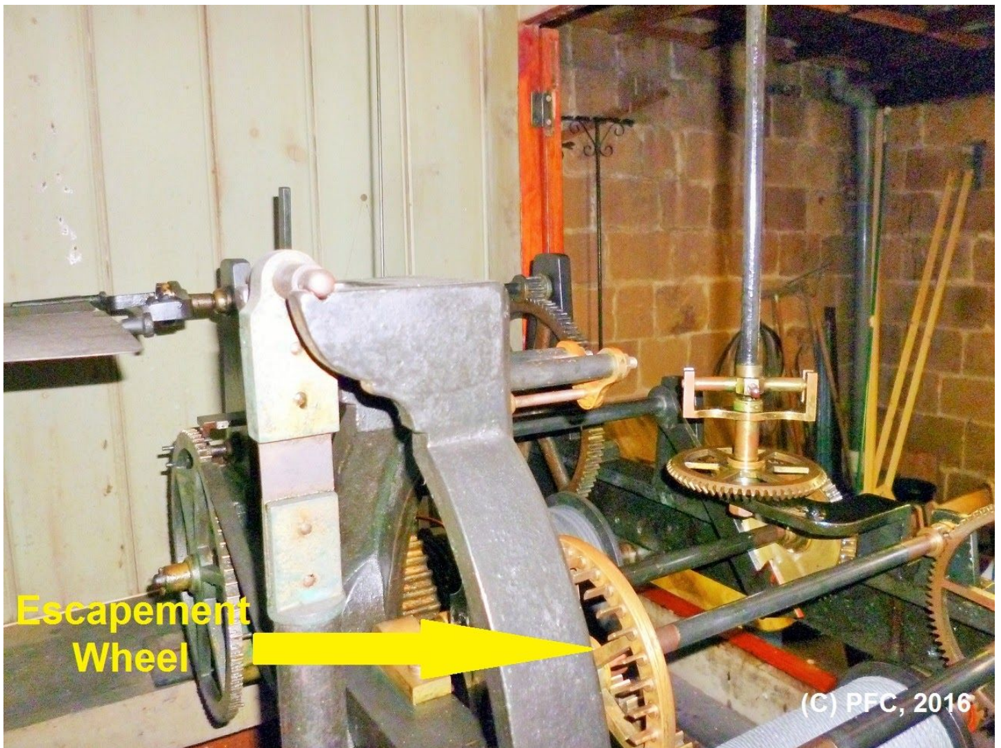
Fig. 7: The escapement wheel as seen from the back of the clock cabinet
