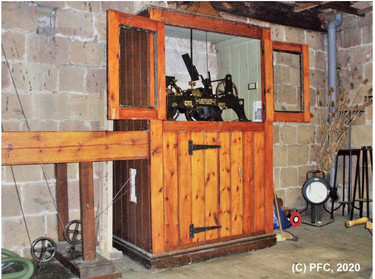
Fig. 4: The large cabinet which protects the clock mechanism
